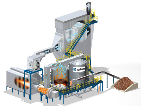
Figure 3: Configuration of 12 MWt Direct Fired Boiler System
